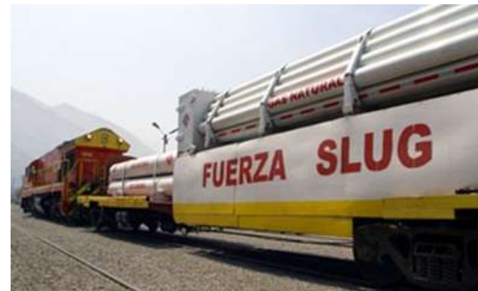
Ferrocarril Central Andino. Perú Locomotive working with CNG
